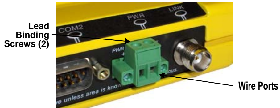
Figure 2-2. Power Connector, Polarity: Left +, Right –
